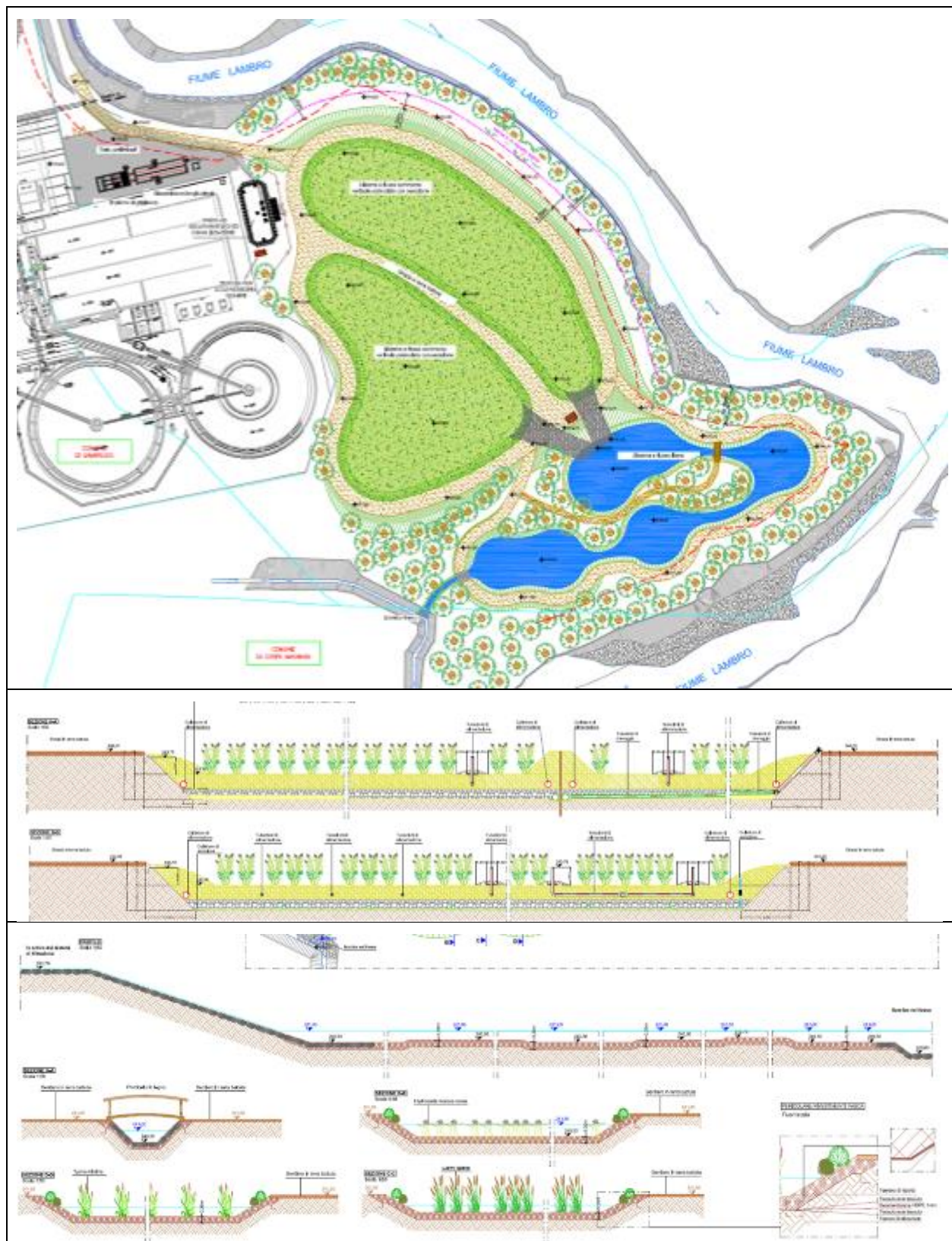
Figure 3: a) general plan of the interventions, b) sections of the submerged flow system and c) sections of the free water surface system as to the definitive project
